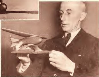
Above is a plastic plane of impregnated spruce plywood and phenol plastic. At the right, Harry Atwood inspects the model of a plastic plane now under construction, which is designed for stratosphere flights. The present war in Europe has spurred interest in the future of plastic planes.
